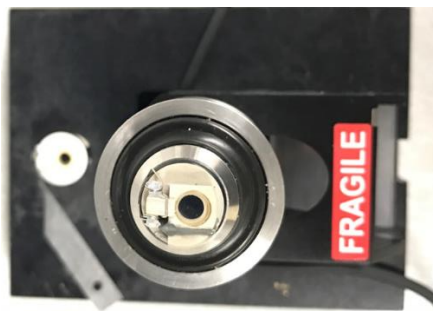
Figure 2.8 Piezo tube scanner with DLFM nosecone attached
