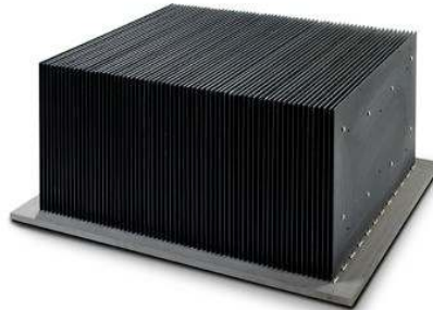
Figure 1.1: Photo of anode package for chlorate production. The electrodes are usually assembled in electrode packages with anodes on one side and cathodes on the other side, or just the anodes in the package using the cell-box as cathode. The latter is the case in this photo. Photo reproduced with permission from Permascand.
