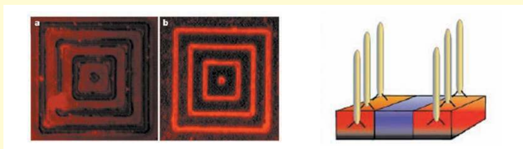
Selection of peptides with semiconductor binding specificity for directed nanocrystal assembly. (a) Control experiment: no phage is present, but primary antibody and streptavidin-tetramethyl rhodamine (TMR) are present. (b) The GaAs-selected phage particle clone specifically recognized the GaAs and not the \text{SiO}_2 surface (courtesy of Angela Belcher, MIT; © 2000 Nature Publishing Group, http://www.nature.com ; reprinted by permission [42]).
