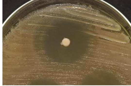
FIGURE 2: Inhibition halo formed around the specimen of glass ionomer cement with silver nanoparticles.
