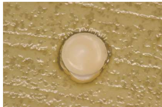
FIGURE 3: Specimen without inhibition halo, representative of Rely X ARC group without silver nanoparticles.
