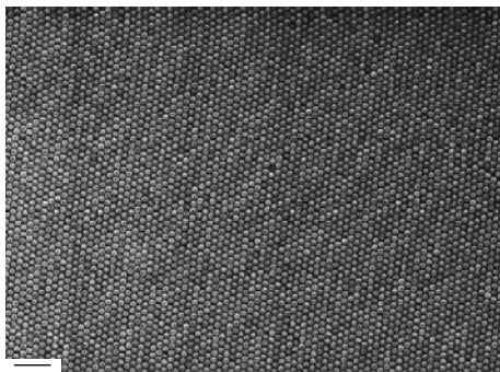
FIGURE 9: SEM micrograph showing large area of self-assembled PS (200 nm diameter) monolayer. The scale bar is 1\ \mu\text{m} . “Reprinted from [70]. Copyright (2009), with permission from Elsevier.”
