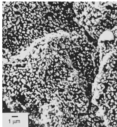
Fig. 1. SEM photomicrograph of ceramic 2A prepared by pyrolysis of 1 at 1200 °C under argon; scale bar: 1 μm (1000 nm).
