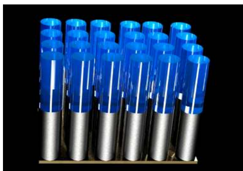
Figure 7. Schematic illustration of Au-PPy nanorods.
