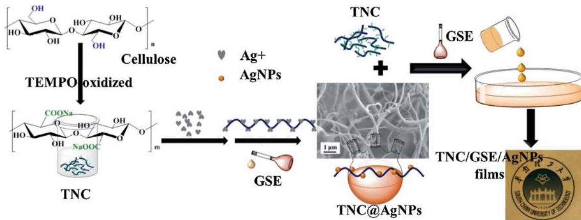
Fig. 10 Preparation of multifunctional TNC/GSE/AgNPs films with antimicrobial and antioxidant activity. Adapted from ref. 114 with permission from Elsevier Ltd, Copyright 2018.
