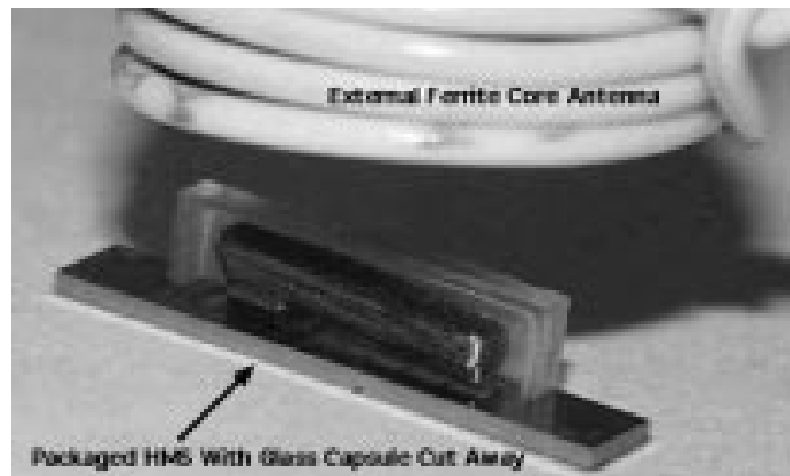
Figure 26 Demo of passive MEMS humidity (moisture) sensor (after T. J. Harpster et al., University of Michigan [49] [50] [51] )
