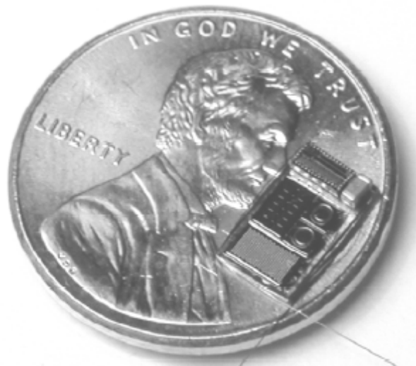
Figure 28 Demo of remote sensing system for relative humidity, pressure, and temperature (after A. D. DeHennis and Khalil Najafi, Fellow, IEEE [52])
