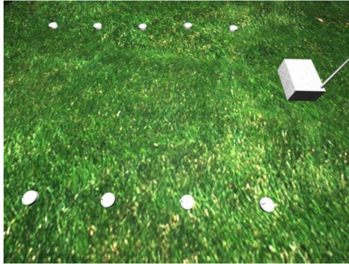
Figure 58 Schematics of distributed wireless sensor network. The distance between sensors (the circular objects in the figure) and data collection center (the rectangular box in the figure) is about 100 ft.
