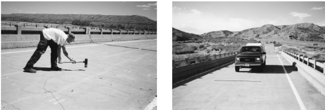
Figure 40 Methods of forced excitation of the Alamosa Canyon Bridge; (left) modal hammer and (right) flatbed truck driving over a wood stud place in the center of the span (after J. P. Lynch et al. [60])
