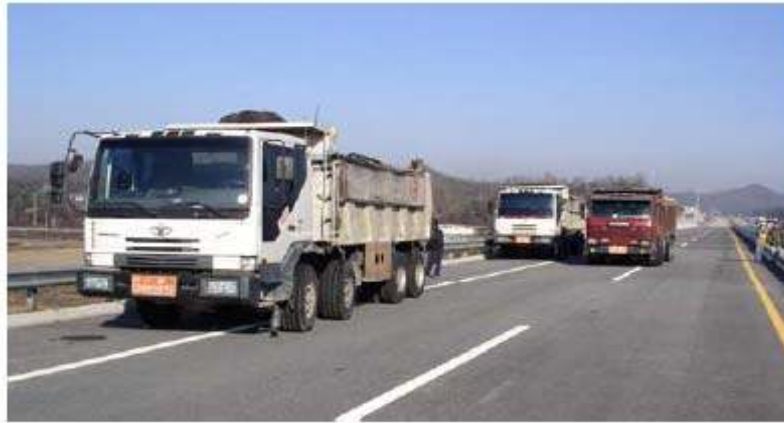
Figure 36 Three trucks (15, 30, and 40 tons) as vibration sources in the Geumdang Bridge (after J. P. Lynch et al. [58] )
