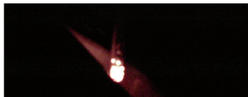
Figure 1. SWNTs in a UHV tube suspended above ( \sim 8 cm) an active microwave source show the white light emission. Room lights were off.
