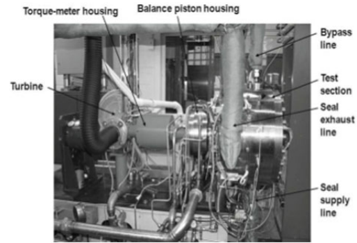
Figure 27.—GRC high temperature, high speed turbine seal test facility (Ref. 12).
