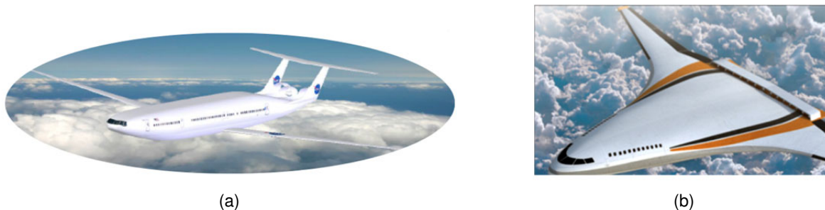
Figure 28.—(a) MIT Double Bubble aircraft concept with propulsors ingesting the fuselage boundary layer (Ref. 2), (b), NASA TurboElectric aircraft concept with propulsors ingesting the blended wing body boundary layer (Ref. 5).
