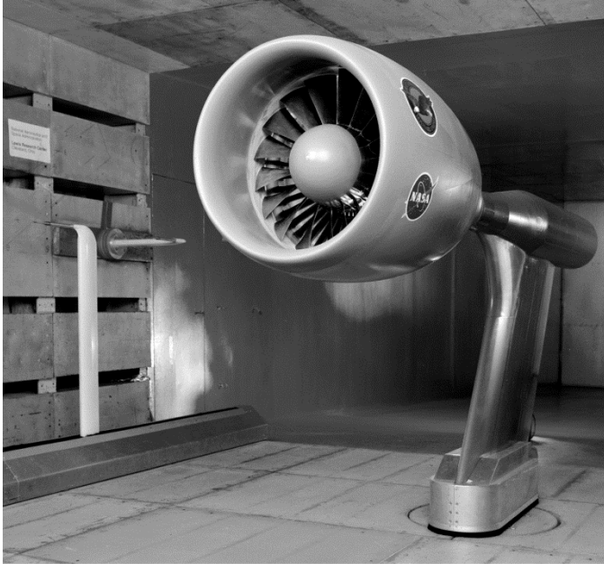
Figure 33.—Advanced Ducted Propulsor (ADP) fan test in 1995.
