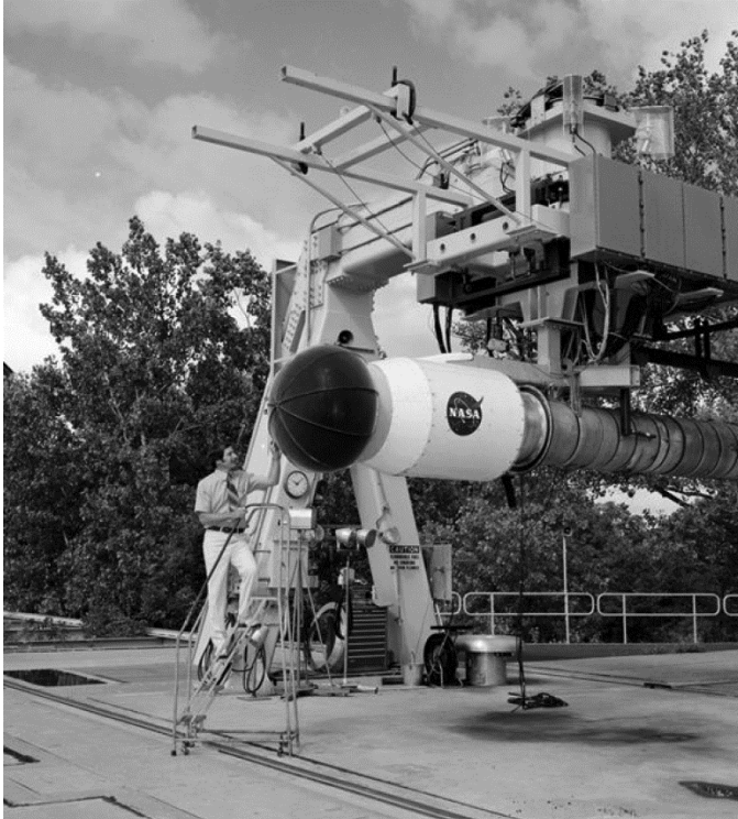
Figure 8.—Outdoor engine facility with JT15D test engine and inflow control device (ICD).
