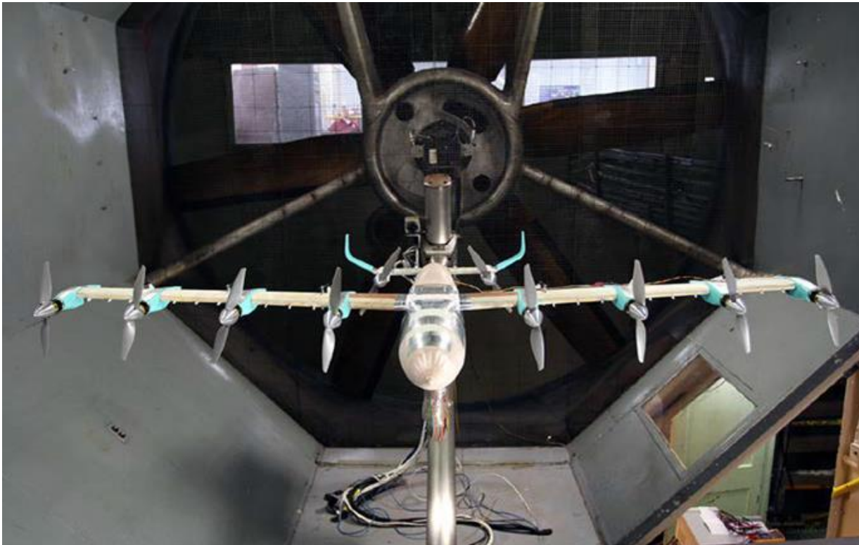
Figure 8. GL-10 28.125% scale tunnel model in NASA Langley's 12-foot Low Speed Wind Tunnel
