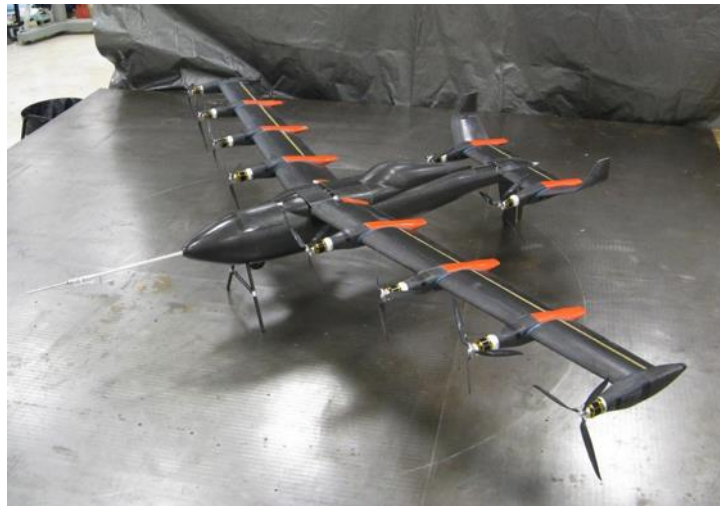
Figure 1. The GL-10 50% scale all-electric prototype aircraft weighing approximately 60 lbs with a 10.5 ft wingspan,
