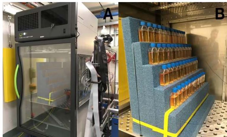
Fig 13. Modified incubator for use in beamline (A) with a holder that can accommodate up to 15 T75 flasks in a 3 \times 5 array or 44 T25 flasks (B).
