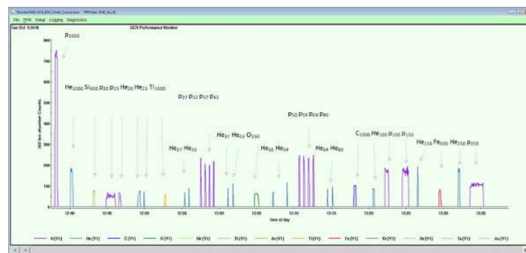
Fig 14. Computer screen shot measuring GCR simulator doses per particle for the 20.8 mGy cycle. GCR, galactic cosmic radiation.
