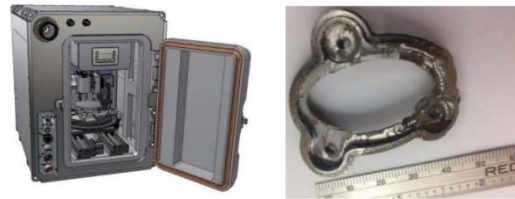
Fig. 10. VULCAN unit from Made in Space. Left image is the rendering of the payload in a double locker and the right image is an example of a metal part produced with the system. Images from Made in Space.
