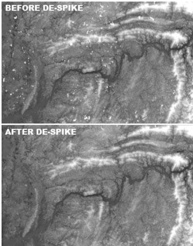
Figure 3. Cloud spike removal from GDEM3 in Gabon, height as brightness.
