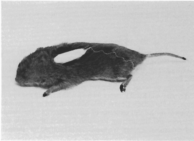
FIG. 2 Meadow vole with a spooling package on her back.
