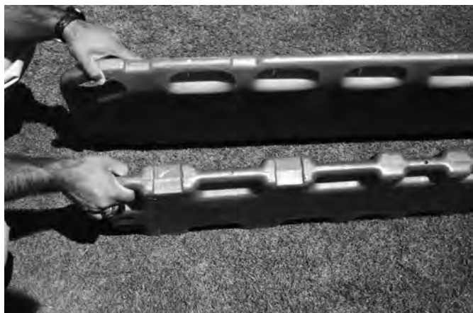
Figure 5. Long spine-board handle designs. The board in the left hand has a beveled bottom, whereas the board in the right hand has recessed handles.
