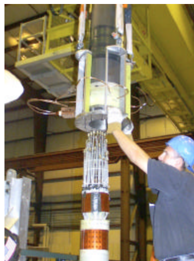
Figure 6- Installation of OH Solenoid
