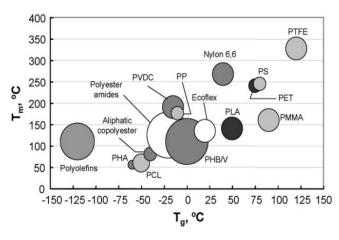
**Figure 5.** Glass transition and melting temperature of PLA with other thermoplastics. (Reproduced with a copyright permission from Tsuji and Ikada [95]).
