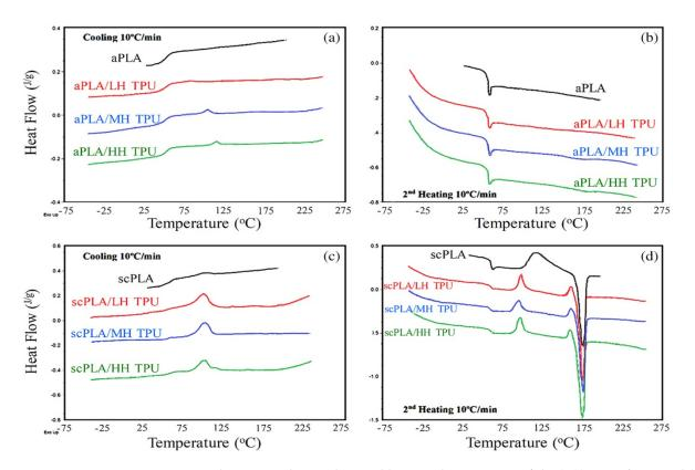
**Figure 9.** The DSC cooling and second heating thermograms of the (**a**,**b**) aPLA/TPU and (**c**,**d**) sc-PLA/TPU blend systems processes [Reproduced with a copyright permission from Nofar et al. [190].
