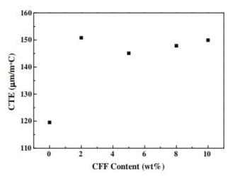
**Figure 7.** Plot of coefficient of thermal expansion for pure PLA and CFF/PLA composites with different CFF contents. (Reproduced with a copyright permission from Cheng et al. [133]).
