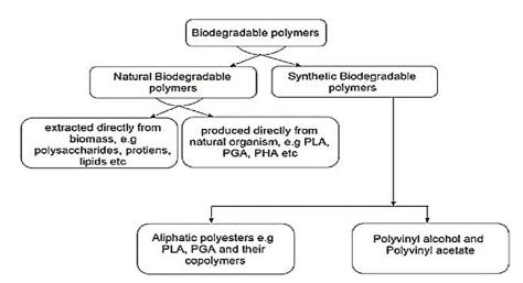
**Figure 2.** The biodegradable classification of polymers constituents in green composites. (Reproduced with a copyright permission from Karande et al. [24]).
