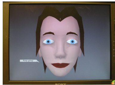
Figure 2: The LCD screen with graphical face used on the robot, shown here with a speech bubble that echos what the robot says (“Keep going!”).
