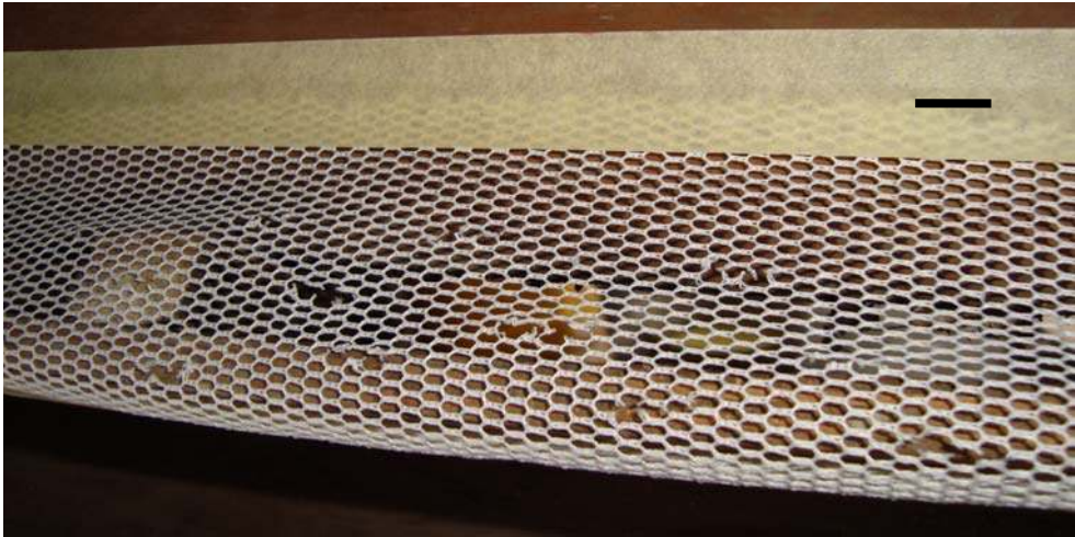
Figure 8.1. A close up of netting attached to the inside of an experimental hut window clearly showing the slits cut to facilitate mosquito passage through the netting; the scale bar (top right) represents 1 cm
