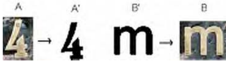
Fig. 11. Principle of image analogies in the context of database increase: A represents the textured and segmented character, A' its binary version. From a binary version of an 'm' in B', the texture is transferred onto B, similar to the analogy between A and A'.
