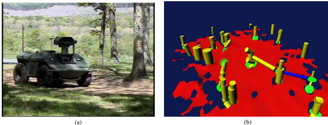
Figure 1: Real-time data processing for scene interpretation. (a) Unmanned vehicle used. (b) Automatically extracted geometric model.
