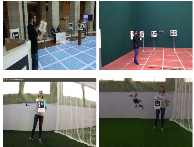
Fig. 12: Here the visual marker interaction is taking place. As can be seen in the bottom left image, the visual algorithm detects the arucos Ids, and perform the commanded tasks.
