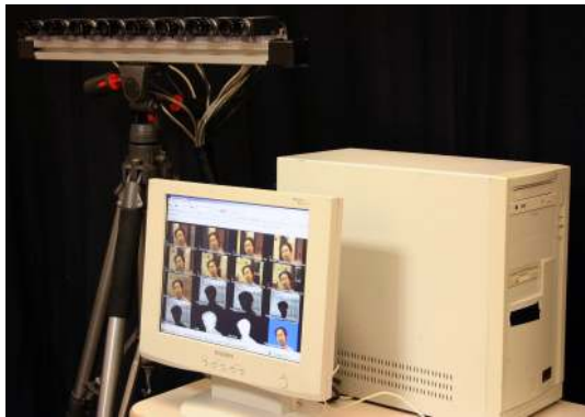
Figure 3: Camera array and real-time system. We use a linear array of 8 video cameras. We can compute alpha mattes at several frames per second at quarter-VGA resolution and generate VGA results offline at about a second per frame.
