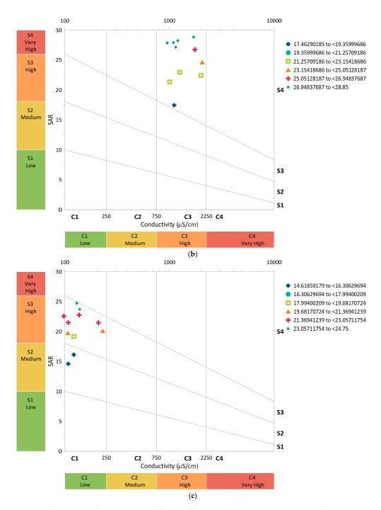
**Figure 5.** The salinity hazard potential from different water sources: (**a**) raw groundwater; (**b**) 0.5 m column depth; (**c**) 1 m column depth ( $V_f$ : 0.0035 L/s; pH: 6.4–12.5; T: 22.6–24.4 °C; n = 8).
