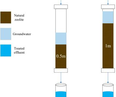
**Figure 6.** Experimental setup (V<sub>f</sub>: 0.0035 L/s; pH: 6.4–12.5; T: 22.6–24.4 °C; *n* = 8).
