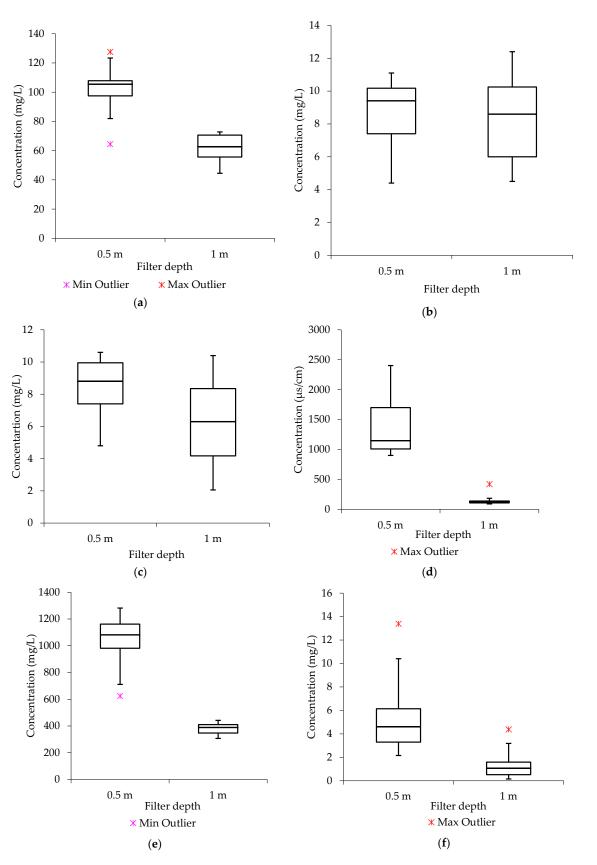
**Figure 2.** Data distribution after treatment (V<sub>f</sub>: 0.0035 L/s; pH: 6.4–12.5; T: 22.6–24.4 °C; n = 8) (a) sodium (Na<sup>+</sup>) (b) calcium (Ca<sup>2+</sup>) (c) magnesium (Mg<sup>2+</sup>) (d) electrical conductivity (EC) (e) total dissolved solids (TDS) (f) potassium (K<sup>+</sup>).
