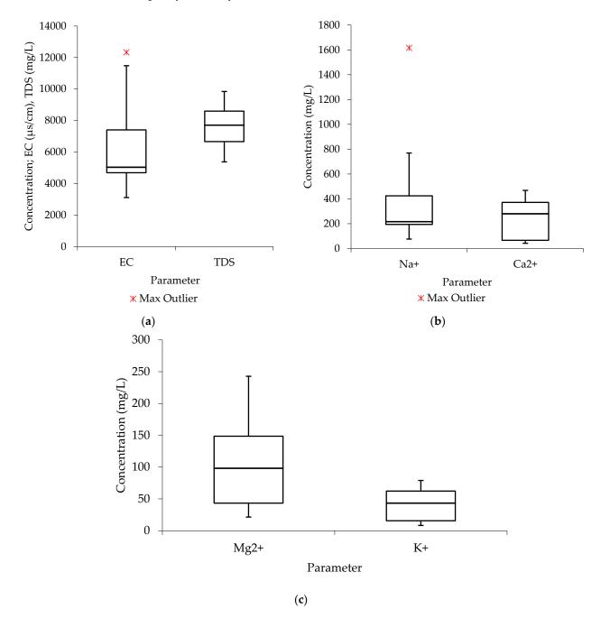
**Figure 1.** Data distribution before treatment (V<sub>f</sub>: 0.0035 L/s; pH: 6.4–12.5; T: 22.6–24.4  $^{\circ}$ C; *n* = 8) (**a**) electrical conductivity and total dissolved solids (**b**) sodium and calcium (**c**) magnesium and potassium.
