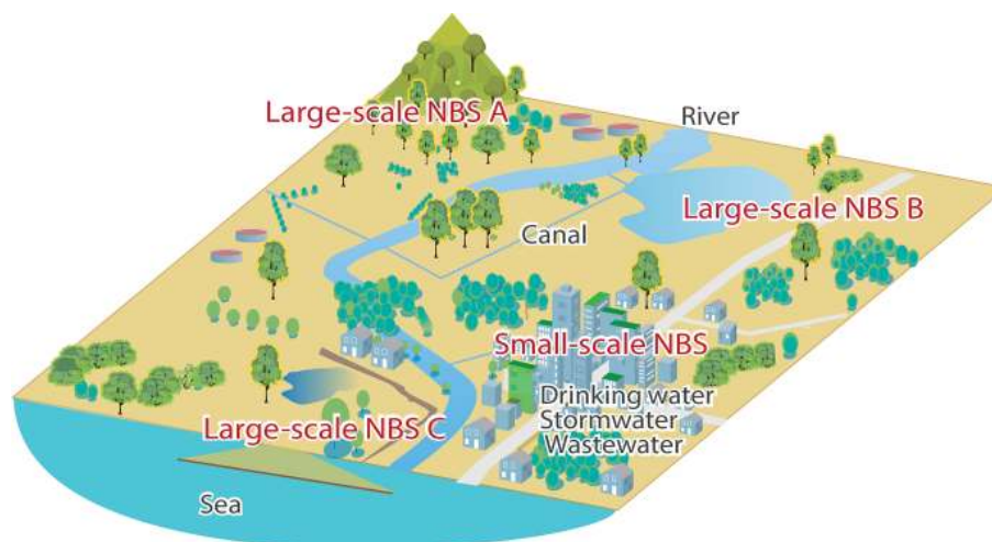
Figure 3. Illustration of large and small-scale nature-based solutions (NBSs). Large-scale NBS A illustrates NBSs in mountainous regions (e.g. afforestation, slope stabilisation, etc.), large-scale NBS B illustrates NBSs along river corridors (e.g. widening river, retention basins, etc.) and large-scale NBS C illustrates NBSs in coastal regions (e.g. sand dunes, protection dikes and walls, etc.). Typical examples of small-scale NBSs are green roofs, green walls, rain gardens, permeable pavements, swales, bio-retention, etc.
