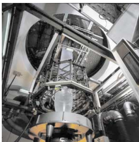
Figure 3. Film blowing with an aliphatic–aromatic copolyester (Ecoflex). Photograph: BASF AG.
