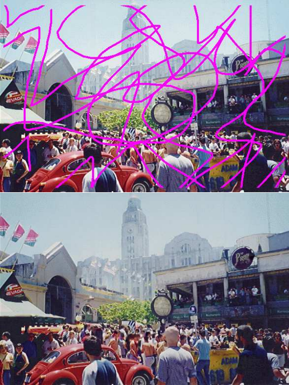
Figure 1. (top) Color photograph with lines obscuring parts of the image, (bottom) Navier-Stokes inpainting restoration of the photograph.
