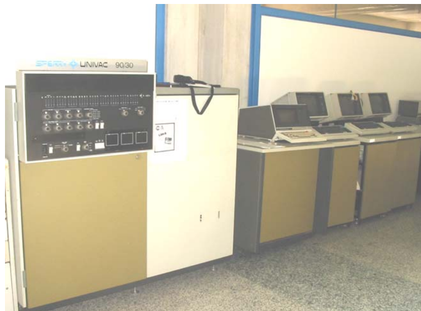
Fig. 2: Some units of a real Univac Sperry 90/30 computer.
