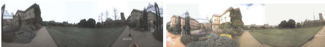
Fig. 7. Example place recognition result generated by FAB-MAP under markedly different lighting conditions. Probability of loop closure is calculated to be 0.9519.
