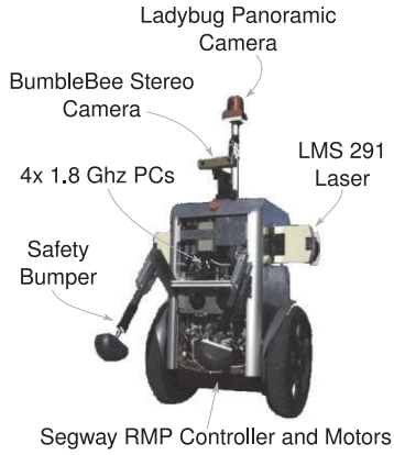
Fig. 2. The results in this paper correspond to data gathered from the modified Segway platform shown above. The vehicle has a sensor payload of two SICK lasers, an XSens inertial sensor, a GARMIN GPS, a Point Grey stereo “Bumblebee” camera and a “Ladybug 2” panoramic camera. It carries four small form factor PCs linked with a Gigabit internal network. Total onboard storage is of the order of 1 TB.
