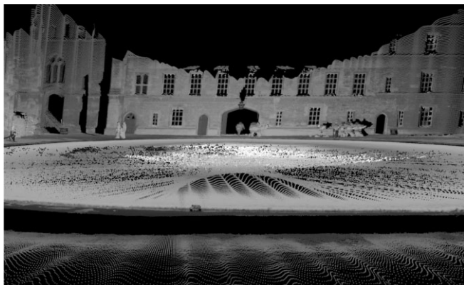
Fig. 22. View of the buildings in the quad of the New College dataset rendered from the 6-DOF estimated trajectory.
