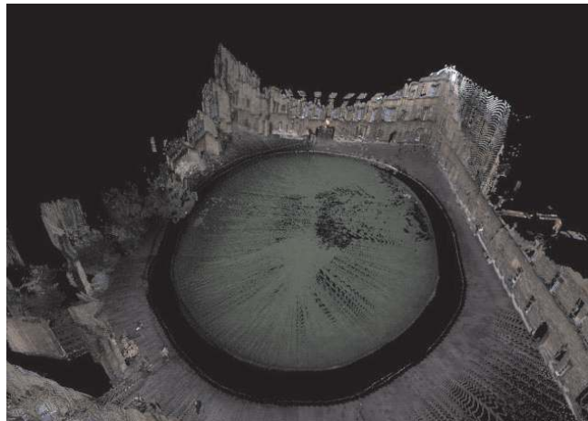
Fig. 23. A view of the New College dataset with color derived from back-projecting laser points into the images taken by the panoramic camera used for loop closure detection.
