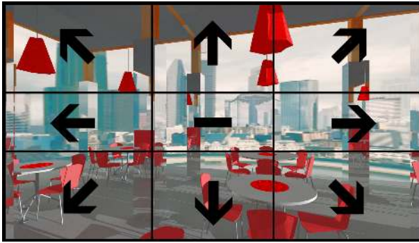
Figure 5: Input actions associated with the gaze directions.
