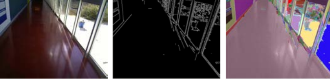
Fig. 11. Example of watershed segmentation using a binary image of marks created with Canny edge detector. Left: Original image. Center: Canny edge detector output. Right: Segmentation result.
