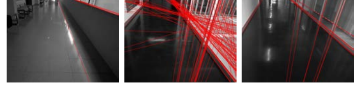
Fig. 10. Example of homogeneous and non homogeneous line distribution. Left and center images show cases of bad distribution. Right image is an example of satisfactory polygonal segmentation due to lines distribution.
