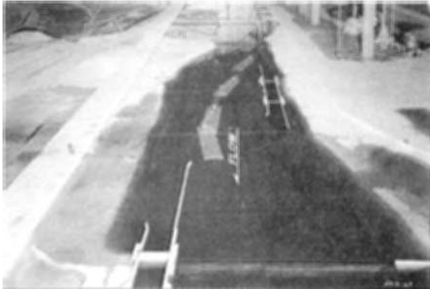
Photo 7. Plan A, looking upstream, discharge 100,000 cfs. Path of downbound tow approaching replacement lock. Note tendency for tow to be moved riverward of guard wall
