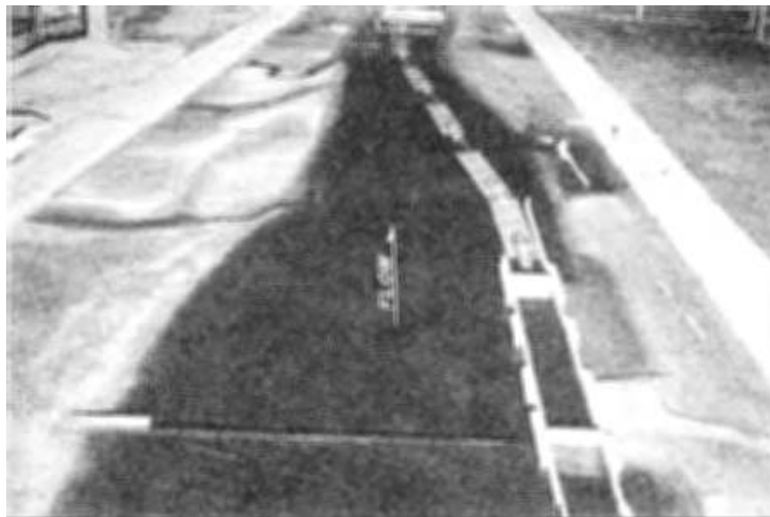
Photo 12. Plan A, looking downstream, discharge 30,000 cfs. Path of downbound tow leaving replacement lock
