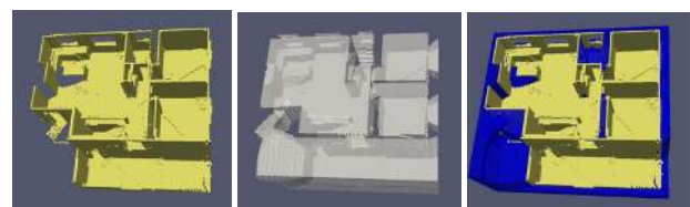
Fig. 5. Reconstructed voxel model with three classes. Left: hard , centre: transparent , right: hard + unknown
