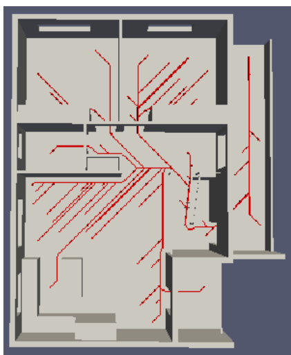
Fig. 3 : Paths to the exit from a number of randomly selected source points
