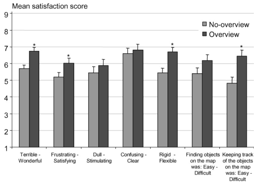
Fig. 6. Satisfaction with the interfaces (for each bar N = 32 ). The figure shows the mean score for the seven satisfaction questions that each subject answered after using each of the two interfaces. Error bars indicate the standard error of the mean. The questions were answered on a 9-point semantic differential going from 1 (lowest score) to 9 (highest score). Significant differences at the .05 level are marked in the figure with an asterisk (*).
