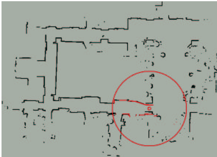
Figure 18: Observed polylines after the robot has completed a tour around our Lab. The polylines shown in light color (red) were captured at the last location of the robot. There is a slight mismatch with polylines sensed at an early stage of the tour.
