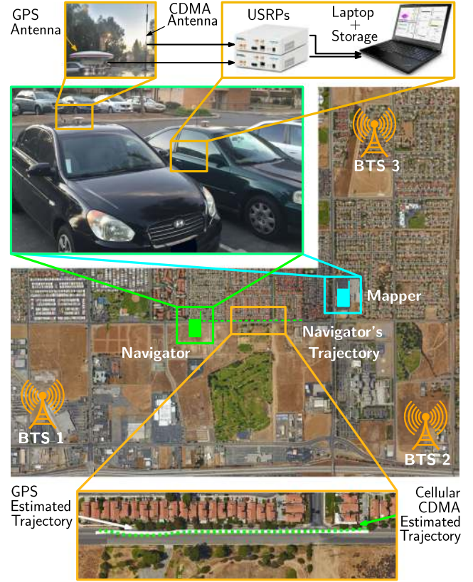
Fig. 6. Experimental hardware setup, navigator trajectory, and mapper and BTS locations for ground experiments. Map data: Google Earth.
