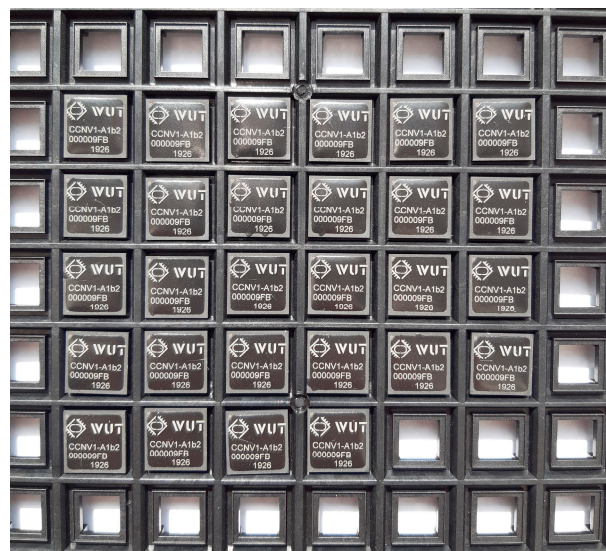
Figure 25. CCNV1-A1 packaged dies.
