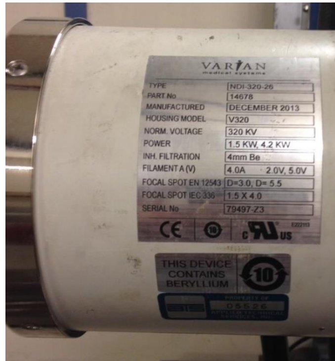
Figure 6.19 NDT-RT-X-ray source details
