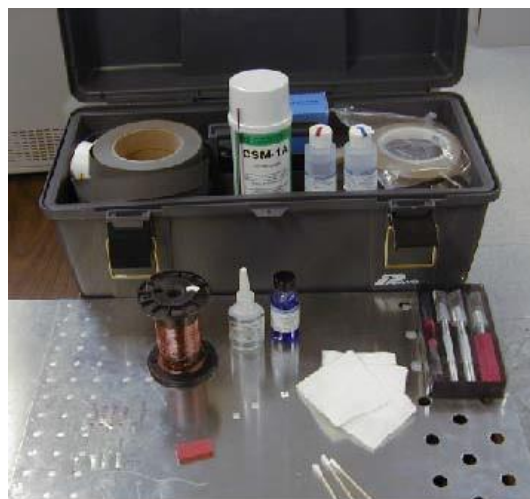
Figure 7.3 The installation kit for strain gages (Giurgiutiu, 2014)
