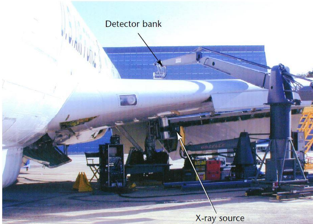
Figure 8.3 NDT-RT for a plane. Adopted from NDT handbook, 3 rd ed.: v 4, RT
