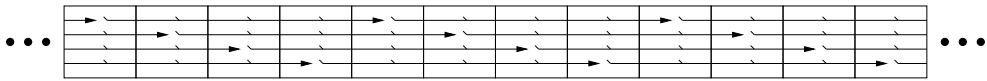
Figure 7.11: Dependencies between sets of 1/R_{\text{IrCC}} = 1.92 IrCC-encoded bits, for a coding memory of L_{\text{IrCC}} = 4 .
