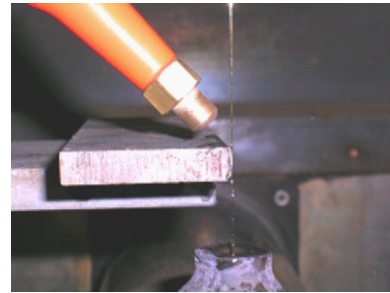
Fig. 1. The delivery of liquid–gas mixture in near dry wire EDM.
