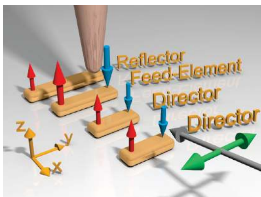
Figure 1. Experimental setup: A Yagi-Uda nanoantenna fabricated on a glass substrate is illuminated by a weakly focused s-polarized (green arrow) laser beam ( \lambda = 1064 nm) under an oblique incident angle (gray arrow). The normal components of the near-fields surrounding the antenna elements (blue and red arrows) can couple to a mode of a sharp AFM tip and are scattered back into the far field.
