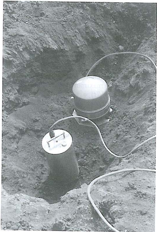
Fig. 2. The deployment at the huddle test station FOS in 1995. While the Guralp CMG3T (bottom) was buried directly the Streckeisen STS-2 (top) was placed on an aluminum plate.
