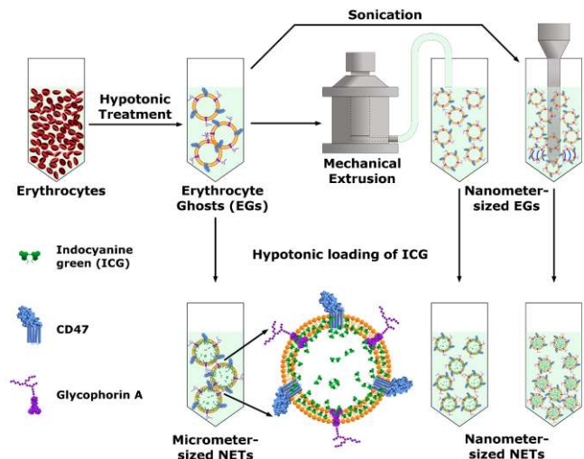
Fig. 1. Schematic of the processes to fabricate micrometer- and nanometer-sized NETs ( \mu NETs and nNETs, respectively). After the formation of micrometer-sized erythrocyte ghosts ( \mu EGs), these particles can be loaded with ICG to form \mu NETs. \mu EGs are mechanically extruded, or sonicated to reduce their size to the nanometer scale before loading with ICG to yield nNETs.
