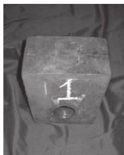
Fig. 4 : ADI Beater head (no shrinkage defect).
