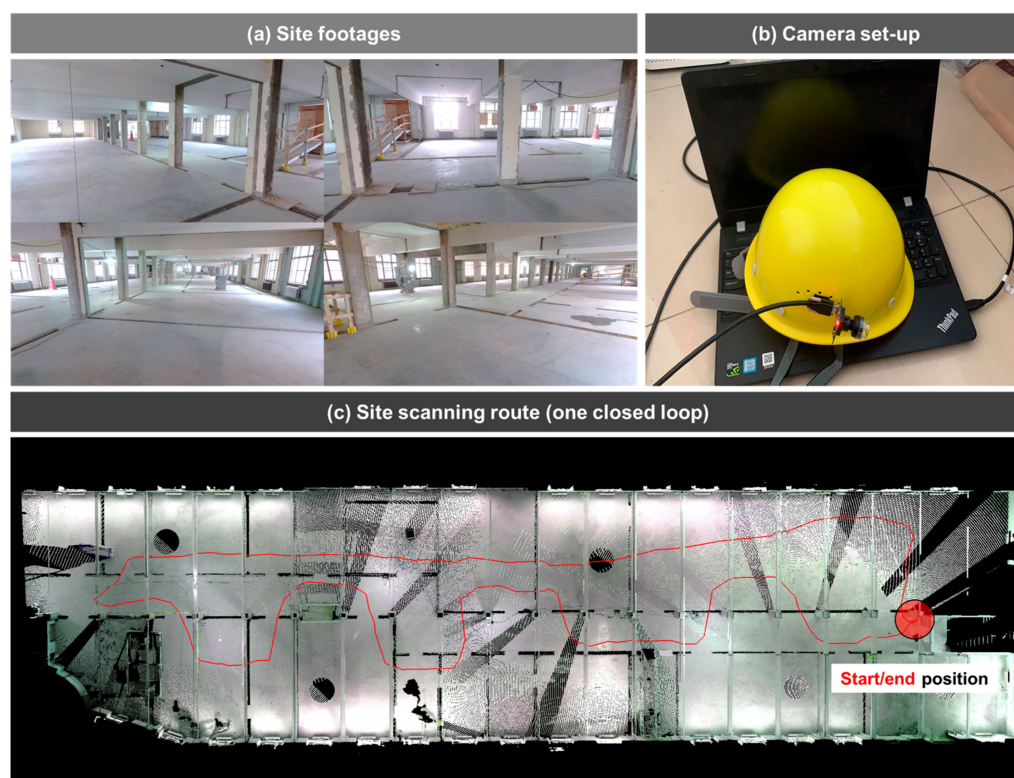
Figure 6. Test setting: site footages and camera set-up.
