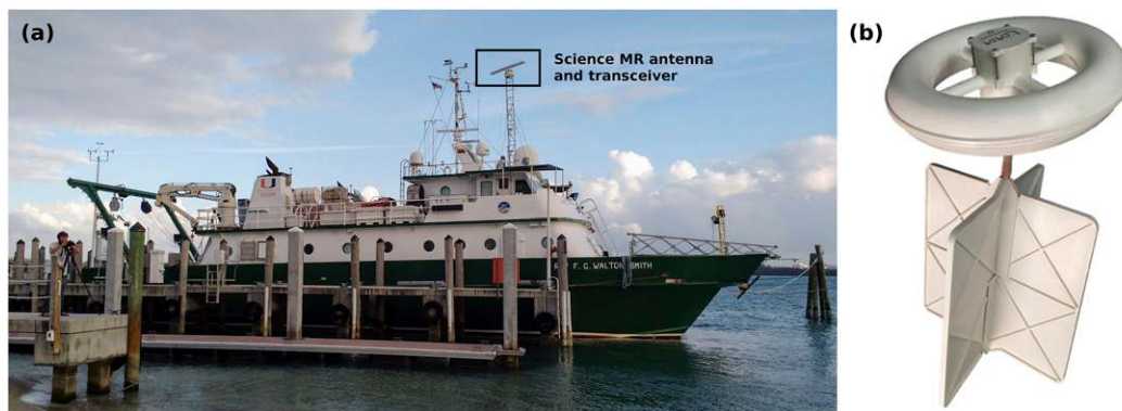
FIG. 2. (a) R/V F. G. Walton Smith at the RSMAS dock in Miami. The HZG MR (black frame) was mounted on a 5-m mast on top of the ship's wheelhouse during LASER. (b) Image of the CARTHE drifter.
